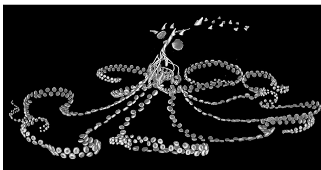
Figure 1. Octopus vulgaris , CT- scan data separating the lead rich glass from the structure
