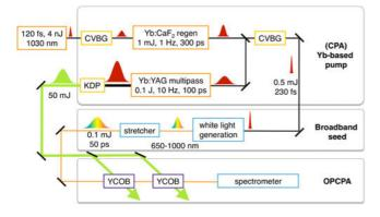
Figure 4. Schematic of diode-pumped OPCPA system.
