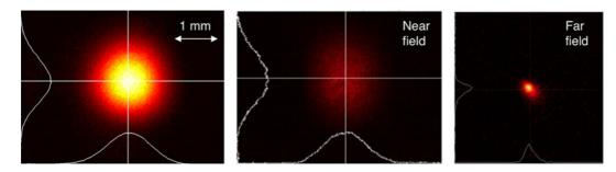
Figure 3. Near-field beam profile at the output of the multipass amplifier (left); near (centre) and far (right) beam profile at the grating compressor output.
