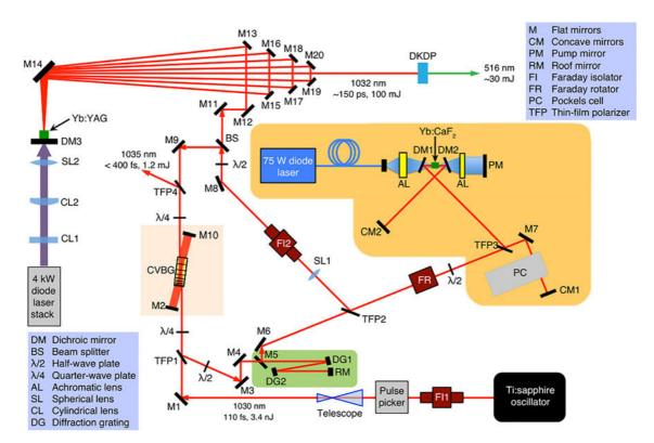
Figure 1. Schematic of the double-stage diode-pumped amplifier, with Yb:CaF<sub>2</sub> regenerative amplifier (orange box, right) and Yb:YAG multipass amplifier (left).
