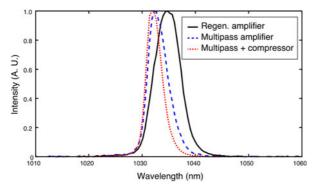
Figure 2. Output spectrum from regenerative amplifier (black), multipass amplifier (blue) and grating compressor (red).
