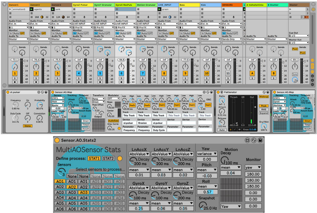
Figure 3. Top: an Ableton Live (AL) session with embedded Max for Live (M4L) patches. Vertical columns represent a bank of input channels as would be found on a traditional audio mixing console, with each channel providing amplitude gain, stereo panning, and routing options. The first three channels (Dancer1/Dancer2/Dancer3) contain pulsar synthesizers coupled to individual sensors worn by three dancers. Additional channels receive audio input from various synthesizers driven by collective mappings. In this figure, the channel Gyro-X-ResPuls is selected, revealing a corresponding audio signal chain in the lower third of the window. The signal chain moves from left to right, starting with a bespoke pulsar synthesizer followed by an instance of the specialized M4L mapping patch (Sensor.AO.Map) designed by the first author. In this case, an aggregate statistical feature, the mean pitch of the three inertial measurement units (IMUs), is selected and mapped to the frequency and duty cycle of the pulsar synthesizer, as well as an “erosion” effect (a short delay line modulated with filtered noise) that is placed further down the signal chain (clipped offscreen in this figure). Bottom: the M4L statistics patch designed by the first author, which allows aggregates of sensor streams to be defined and evaluated statistically and subsequently used as control signals by mapping patches.
