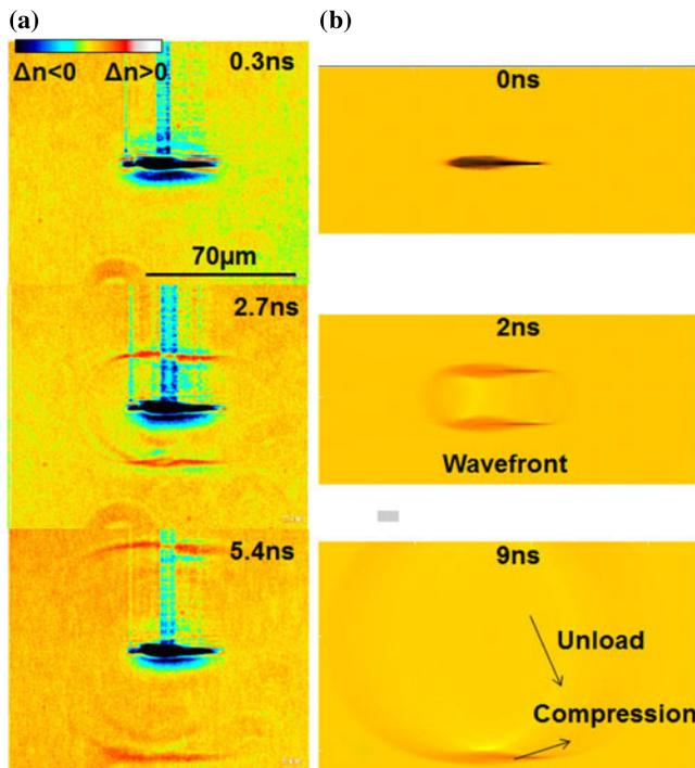
**Figure 6.** Photo-acoustic dynamics in fused silica observable at different time delays (a) in experimental time-resolved PCM images of evolving pressure waves and (b) in photo-acoustic simulation for a moderate energy input of  $4 \mu\text{J}$ . Pulse duration is 2 ps for (a) and 150 fs for (b). The laser pulse is coming from the left. The color bar relates to evolving relative positive and negative refractive index changes.
