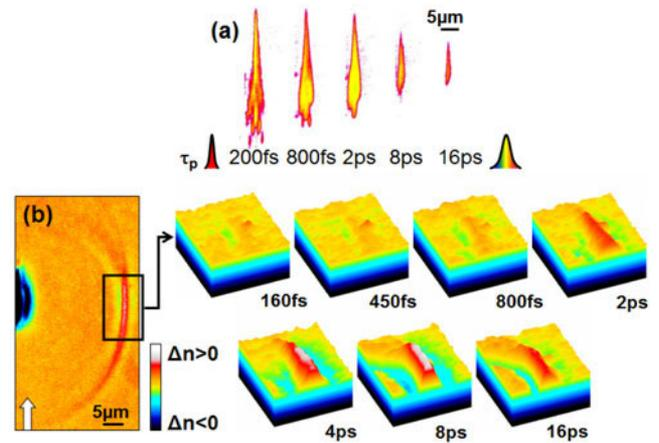
**Figure 7.** (a) Excitation increase (absorption maps in false colors) upon irradiation with pulses of increasing duration. (b) Pressure wave magnitude dependence in fused silica on the input pulse duration for an energy of  $4 \mu\text{J}$ . The color bar indicates relative positive and negative transient refractive index changes associated to thermomechanical phenomena.
