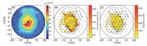
FIGURE 8. (a) Example of closed-field line geometry featuring quasi-circular flux surfaces. Also shown is the time-averaged profile of the ion saturation current density. From HEXTIP data: 2D poloidal distribution of (b) structure trajectories, average velocity field and (c) number of structures detected. Contours of the time-averaged ion saturation current density profile are shown at 25% (outermost), 50% and 75% of the maximum.
