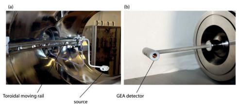
FIGURE 3. Experimental setup for suprathermal ion studies: (a) suprathermal ion source installed on a toroidal moving rail inside TORPEX and (b) gridded energy analyzer installed on a 2D poloidal moving system.
