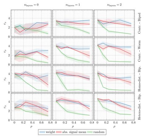
**Figure 10.** Median, lower quartiles, and upper quartiles of re-assessment velocity  $v_x$  vs. pruning rate  $\rho$  averaged across re-assessment terrains for different pruning criteria, VSR controller architectures, VSR morphologies, and ANN topologies.
