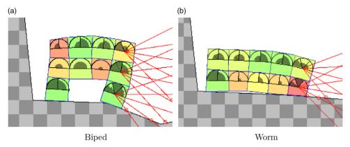
Figure 1. Frames of the two VSR morphologies used in the experiments. The color of each voxel encodes the ratio between its current area and its rest area: red indicated contraction, yellow rest state, and green expansion. The circular sector drawn at the center of each voxel indicates the current sensed values: subsectors represent sensors and are, where appropriate, internally divided into slices according to the sensor dimensionality m. The rays of the vision sensors are shown in red.
