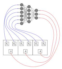
**Figure 2.** A schematic representation of the centralized controller for a  $3 \times 1$  VSR with two sensors in each voxel. Blue and red curved arrows represent the connection of the ANN with inputs (sensors) and outputs (actuators), respectively.
