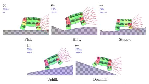
Figure 9. Different types of terrains employed for measuring VSR adaptability.
