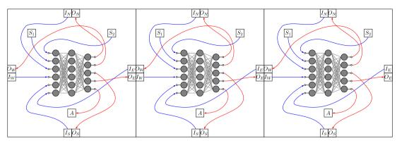
Figure 3. A schematic representation of the distributed controller for a  $3 \times 1$  VSR with two sensors in each voxel and  $n_c = 1$  communication channel per side. Blue and red curved arrows represent the connection of the ANN with inputs (sensors and input communication channels) and outputs (actuator and output communication channels), respectively.
