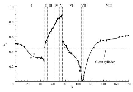
Figure 8. Variation of the non-dimensional amplitude of oscillations  $A^*$  with the wire angular position  $\theta$ . The horizontal dashed line indicates the oscillation amplitude of the clean cylinder, which has the value of  $A^* = 0.44$ . The uncertainty is the same for all cases and is marked on the plot for some data points as a reference.
