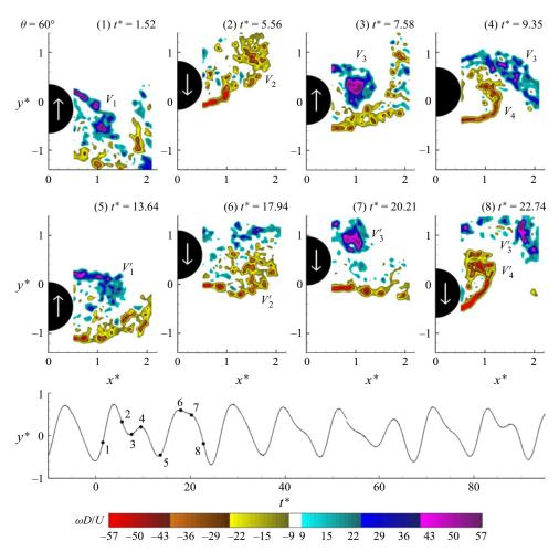
Figure 14. Contours of instantaneous normalized vorticity  $(\omega D/U)$  for the wire angular position  $\theta=60^\circ$  (from range IV) along with the time traces of the cylinder displacement. The minimum absolute value and the incremental value of contour levels are:  $[|\omega|D/U]_{min}=9$  and  $\Delta(\omega D/U)=1.15$ .
