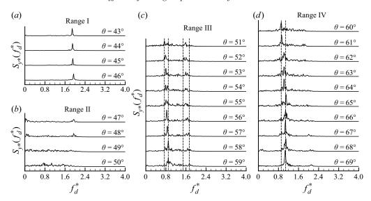
Figure 7. Autospectral density of the cylinder displacements,  $S_{y^*}(f_d^*)$ , for select locations of the wire in: (a) range I  $(0^\circ \le \theta < 47^\circ)$ , (b) range II  $(47^\circ \le \theta < 51^\circ)$ , (c) range III  $(51^\circ \le \theta < 60^\circ)$  and (d) range IV  $(60^\circ \le \theta < 70^\circ)$ .
