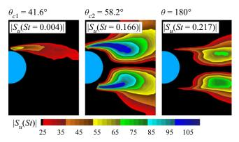
Figure 2. Contours of autospectral density of the streamwise velocity fluctuations at the specific Strouhal number value indicated in the inset for the stationary cylinder fitted with the surface wire at the first  $\theta_{c1}$  and second  $\theta_{c2}$  critical angles, and at  $\theta=180^\circ$  (representing the clean cylinder). Minimum and incremental values of the contours are  $[|S_u(St)|]_{min}=25 \text{ mm s}^{-1}$  and  $\Delta[|S_u(St)|]=2.5 \text{ mm s}^{-1}$ .
