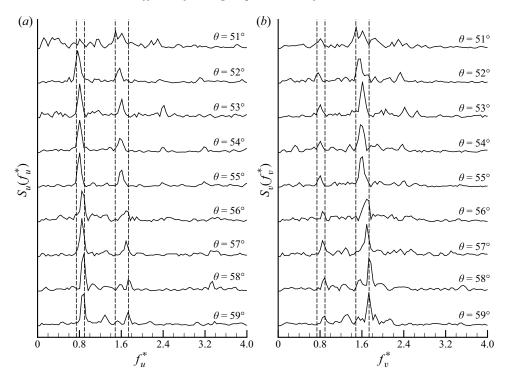
Figure 22. Frequency spectrum of velocity signals at a point with maximum value of spectral magnitude for wire angular positions of range III  $((51^{\circ} \le \theta < 60^{\circ}))$ . Existence of two distinct dominant frequencies is depicted for both: (a) the streamwise velocity component u and (b) the transverse velocity component v.
