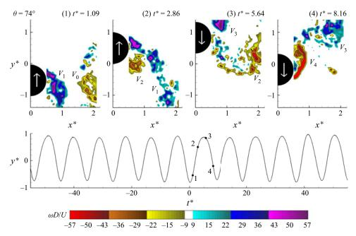
Figure 15. Contours of instantaneous normalized vorticity  $(\omega D/U)$  for the wire angular position  $\theta = 74^{\circ}$  (from range V) along with the time traces of the cylinder displacement. The minimum absolute value and the incremental value of contour levels are:  $[|\omega|D/U]_{min} = 9$  and  $\Delta(\omega D/U) = 1.15$ .
