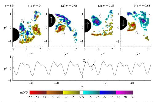
Figure 13. Contours of instantaneous normalized vorticity  $(\omega D/U)$  for the wire angular position  $\theta=53^\circ$  (from range III) along with the time traces of the cylinder displacement. The minimum absolute value and the incremental value of contour levels are:  $[|\omega|D/U]_{min}=9$  and  $\Delta(\omega D/U)=1.15$ .
