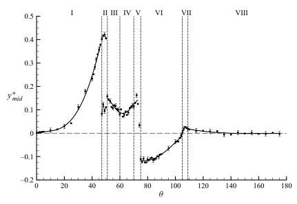
Figure 9. Variation of the mid-position  $y_{mid}^*$  of the oscillating cylinder with the wire angular position. The positive direction of the vertical axis corresponds to the wire side of the cylinder.  $y_{mid}^* = 0$  is the equilibrium state in still water for both clean and tripped cylinders. The horizontal dashed line indicates the mid-position of oscillation for the clean cylinder. The uncertainty is the same for all cases and is marked on the plot for some data points as a reference.
