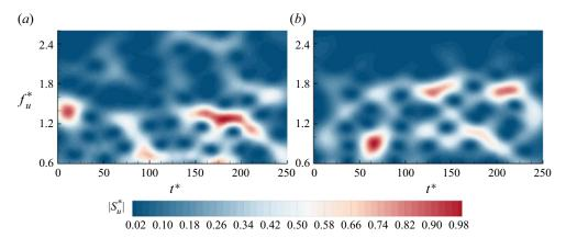
Figure 12. Time–frequency spectrogram of the streamwise velocity component for: (a) the stationary cylinder with the wire at the first critical angle ( $\theta_{c1} = 42^{\circ}$ ), and (b) the oscillating cylinder with the wire placed at  $\theta = 48^{\circ}$  (within the angular range II). The magnitude of spectra  $|S_u^*|$  is normalized based on the maximum value in the entire period, and the incremental value of the contour levels is  $\Delta[|S_u^*|] = 0.02$ .
