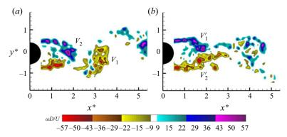
Figure 17. Contours of instantaneous normalized vorticity  $(\omega D/U)$  for the wire angular position  $\theta=107^\circ$  (from range VII) with random switching of the vortex shedding mode between (a) Mode I and (b) Mode II. The minimum absolute value and the incremental value of contour levels are:  $[|\omega|D/U]_{min}=9$  and  $\Delta(\omega D/U)=1.15$ .
