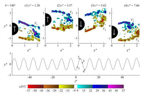
Figure 19. Contours of instantaneous normalized vorticity  $(\omega D/U)$  for the wire angular position  $\theta=140^\circ$  (from range VIII) along with the time traces of the cylinder displacement. The minimum absolute value and the incremental value of contour levels are:  $[|\omega|D/U]_{min}=9$  and  $\Delta(\omega D/U)=1.15$ .
