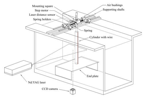
Figure 1. Three-dimensional sketch of the experimental set-up.
