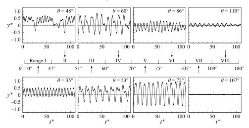
Figure 4. Time traces of the cylinder position for the application of the wire at different angular locations on the cylinder surface. The axis of angular values, where the range divisions are shown, is not to scale.
