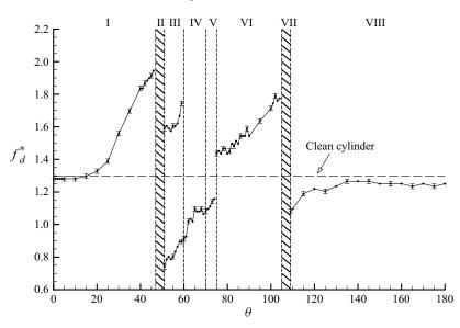
Figure 5. Variation of the frequency of cylinder oscillations in non-dimensional form  $(f_d^* = f_d/f_n)$  with the wire angular position. The horizontal dashed line indicates the non-dimensional frequency of the oscillation motion for the clean (untripped) cylinder.
