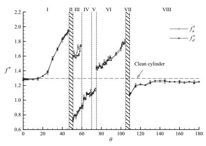
Figure 21. Variation of the dominant frequency of the oscillation motion  $f_d^*$  and the dominant frequency of the streamwise velocity fluctuations  $f_u^*$  with the wire angular position  $\theta$  for the oscillating wire-fitted cylinder. The horizontal dashed line marks both the oscillation frequency and the dominant frequency of streamwise velocity signals for the clean cylinder undergoing VIV under the same conditions.
