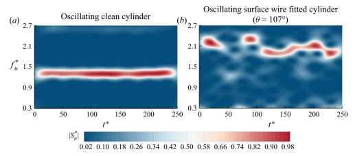
Figure 18. The short-time Fourier transform (STFT) of the streamwise velocity for: (a) the clean cylinder and (b) the cylinder fitted with the wire at  $\theta = 107^{\circ}$ . The magnitude of the velocity spectra is normalized based on the maximum value in the entire period. The normalized frequency resolution is 0.02 and the temporal resolution is 0.21 s. The incremental value of contour levels is  $\Delta[|S_u^*|] = 0.02$ .
