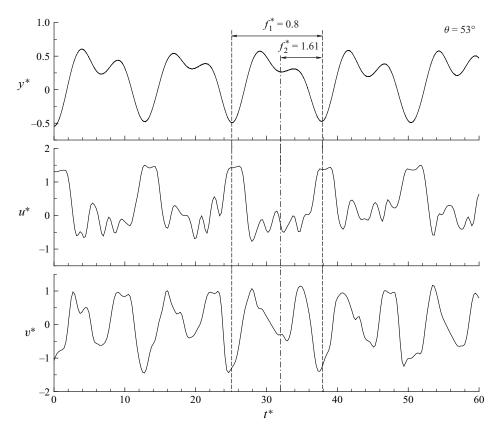
Figure 23. Time traces of displacement of the cylinder  $y^*$ , the streamwise velocity component  $u^*$  and the transverse velocity component  $v^*$  for the wire angular location of  $\theta = 53^\circ$  (from range III). The period of the non-dimensionalized time is the same for all plots. One cycle of oscillation motion is marked between the two vertical dashed lines.
