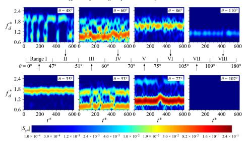
Figure 6. Time–frequency spectrogram of the cylinder oscillations for having the wire at different angular locations on the cylinder surface. The axis of angular values, where the range divisions are shown, is not to scale.
