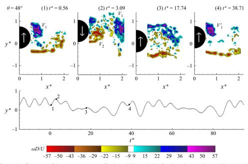
Figure 11. Contours of instantaneous normalized vorticity  $(\omega D/U)$  for the wire angular position  $\theta=48^\circ$  (from range II) along with the time traces of the cylinder displacement. The minimum absolute value and the incremental value of contour levels are:  $[|\omega|D/U]_{min}=9$  and  $\Delta(\omega D/U)=1.15$ .
