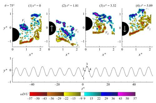
Figure 16. Contours of instantaneous normalized vorticity  $(\omega D/U)$  for the wire angular position  $\theta = 75^{\circ}$  (from range VI) along with the time traces of the cylinder displacement. The minimum absolute value and the incremental value of contour levels are:  $[|\omega D/U]_{min} = 9$  and  $\Delta(\omega D/U) = 1.15$ .
