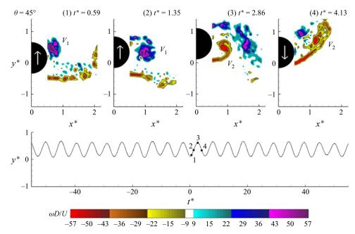
Figure 10. Contours of instantaneous normalized vorticity  $(\omega D/U)$  for the wire angular position  $\theta=45^\circ$  (from range I) along with the time traces of the cylinder displacement. The minimum absolute value and the incremental value of contour levels are:  $[|\omega|D/U]_{min}=9$  and  $\Delta(\omega D/U)=1.15$ .
