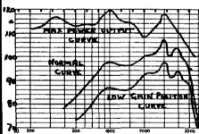
Frequency Response 500 - 5000 cps. Maximum Amplification (at 3000 cps) 46 dB. Maximum power output (1000 cps) 120 dB.
