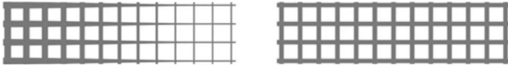
Figure 1. A heterogeneous (left) and homogeneous (right) lattice structures (Tang et al., 2019)
