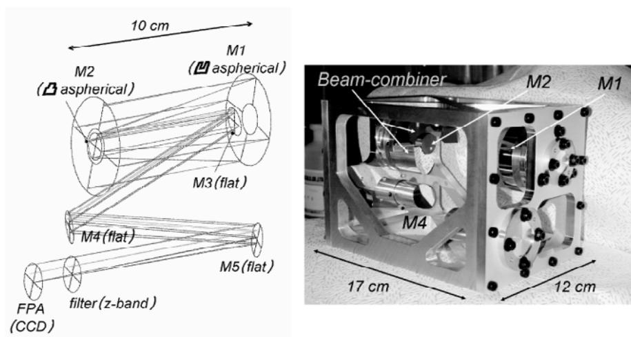
**Figure 1.** *Left:* Optical layout of Nano-JASMINE telescope. A beam-combiner that should appear around the M2 is omitted here. *Right:* Assembled proto-model of the telescope. All parts are figured out of aluminum alloy except the gold coat on the optical reflecting surfaces.
