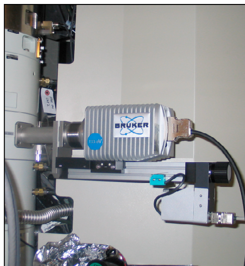
Fig. 1. Bruker-AXS silicon drift detector installed on JEOL 2200FS aberration-corrected STEM/TEM.
