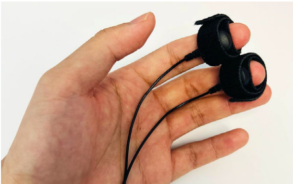
Figure 2. GSR wired electrodes. The sensor consists of two wired electrodes attached to the fingers and collects data at a sampling rate of 10 Hz.
