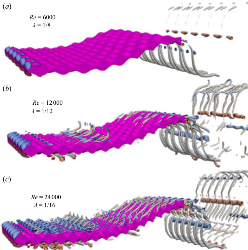
Figure 7. Flow structures of plates at  $Re = 6, 12$  and  $24 \times 10^3$  visualised by the same Q-criterion. The surface topographies, defined by  $\lambda = 1/8, 1/12, 1/16$ , correspond to the enstrophy peaks discussed in § 3.4. The time evolution of these three flow fields are available as supplementary movies, available at <https://doi.org/10.1017/jfm.2023.703>.
