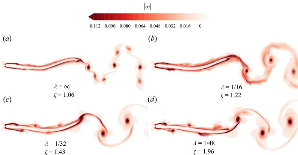
Figure 5. The change in vorticity magnitude with roughness wavelength. All instances are taken at the same cycle time ( $t = 0.1$ ) and show the spanwise-averaged vorticity magnitude: (a) a smooth plate; (b–d) rough plates defined by decreasing  $\lambda$ .
