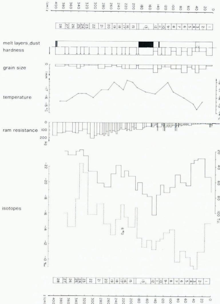
Fig. 3. Snow characteristics and isotopes in the snowpit. 1–28 = layer numbers.
