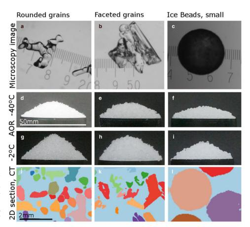
**Fig. 1.** Investigated snow samples in the columns; from left to right: RG, FC, IBS. In the rows: 1 (a)–(c) Microscope image of one representative grain (scale in mm). In row 2 (d)–(f) exemplary heaps showing the angle of repose (AOR) at  $-40^{\circ}$ C (RG at  $-30^{\circ}$ C) and in row 3 (g)–(i) heaps at  $-2^{\circ}$ C. Row 4 (j)–(l) shows 2D section of 3D  $\mu$ CT images after binary and watershed segmentation (same scale).
