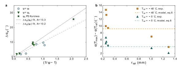
**Fig. 6.** (a) Shape contribution  $\Delta \alpha_{\psi}$  of experiments (Eqn (7)) and model ( $A(1/\psi - 1)$ ) for both shape parameters,  $\psi_s$  and  $\psi_r$  (b) Cohesional contribution  $\Delta \alpha_c$  of experiments against  $\mu$ CT-derived particle radius  $r_{opt}$ : orange squares show the maximum *T*-induced change and green triangles show the change between the two highest temperatures; in the model, the cohesional contribution only depends on *T*.
