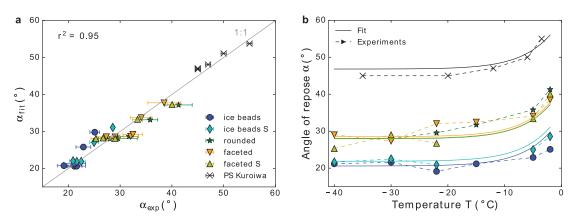
Fig. 5. Comparison of experiments and model fit (Eq (6), with  $\psi = \psi_s$ ), in (a) as a scatter plot, and in (b) against temperature.
