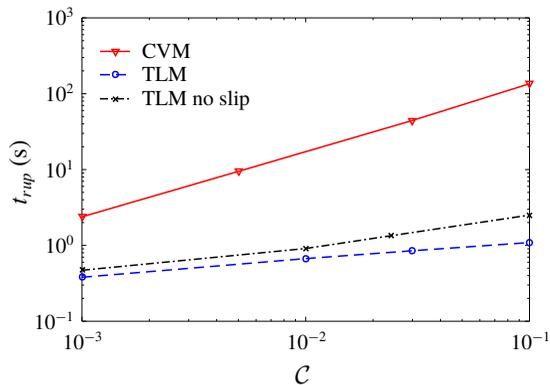
FIGURE 1. Dimensional rupture time  $t_{rup}$  as a function of the dimensionless surface tension  $C$ . The dotted lines are predictions of the two-layer model (TLM) with and without slip on the substrate. This replaces the original figure 12 in Dey *et al.* (2019).
