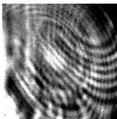
Fig. 1. Ronchigram of graphite 3.4 Å fringes recorded soon after the beam was first brought up through the new column.
