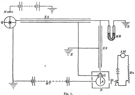
A. Anode of Photo-electric Cell; AM. Ammeter in Lighting Circuit; B. Light-tight box; E. Earth; ES. Electrostatic Shield; G. Guard Ring; HT. High Tension Battery; HR. High Resistance; L. Lamp; N. Electrometer needle; Q. Quadrant Electrometer; Rh. Rheostat; S. Brass Shutter.
