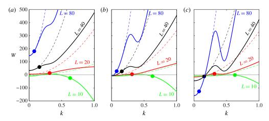
FIGURE 7. (Colour online) Effect of small A blowing and suction with wavelength L on the critical Reynolds number for perturbations of underlying wavenumber k as measured through the weighted-residual results for W, with C=0.05. The filled circles on each curve mark the point where  $k=2\pi/L$ . The dashed lines show the long-wave asymptotic estimate (5.16). (a)  $\theta=\pi/4$ , (b)  $\theta=\pi/2$ , (c)  $\theta=3\pi/4$ .
