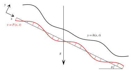
FIGURE 1. (Colour online) Sketch of flow domain showing coordinate system. We consider a fluid layer with mean height  $h_s$ , bounded along y = 0 by a rigid planar wall inclined at angle  $\theta$  to the horizontal, and at y = h(x, t) by a free surface. Fluid is injected through the wall, and so the normal velocity at the wall is given by the prescribed function v = F(x, t).
