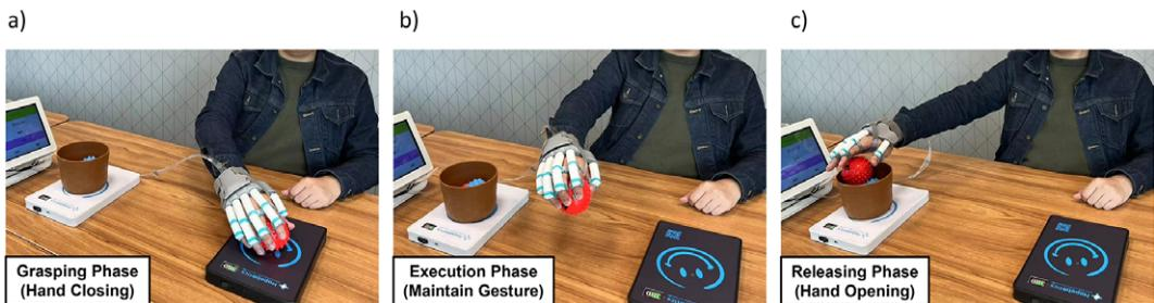
**Figure 3.** Example of task training process for moving objects task (ball,  $d = 80$  mm). (a) Patient wearing a soft robotic hand approaches the task board (black), and activates interactive grasp mode for ball grasping, (b) Patient's hand leaves the task board (black), soft robotic hand maintains grasping assistance during the task execution phase.
