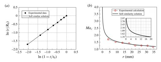
FIGURE 6. (Colour online) (a) Logarithmic plot of the shock position as a function of time with a fitted line of the self-similarity solution for  $Ma_0 = 1.17$ . (b) Experimental measurements and self-similarity fitted line showing the variation of shock Mach numbers as a function of the position. The inset shows a magnification of the fitted line within r = 20 mm.
