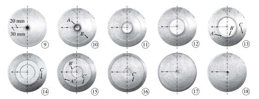
FIGURE 7. Sequence of schlieren images showing the propagation of shock waves in observation region for  $Ma_0 = 1.17$ , which is a continuation of figure 5. Again, the frame rate of the high-speed video camera is 105 000 f.p.s. corresponding to a time interval between two consecutive frames of about 9.52  $\mu$ s. The number in the lower right corner of each image represents the sequence of the images. The locations of 20 and 30 mm away from the focal point are marked.
