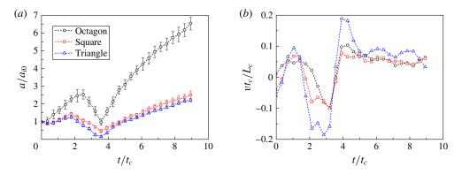
FIGURE 19. (Colour online) Quantitative data showing the normalized amplitudes  $a/a_{i0}$  (*a*) and corresponding normalized growth rates  $vt_c/L_c$  (*b*) of the polygonal gas cylinder versus the dimensionless time  $t/t_c$ .
