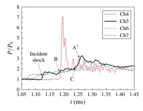
FIGURE 8. (Colour online) Experimental pressure histories at transducers Ch4–Ch7 mounted on the top wall of the test section. The arrival of different shock waves at transducer Ch5 (30 mm from the focal point, as indicated in figure 7) are highlighted.
