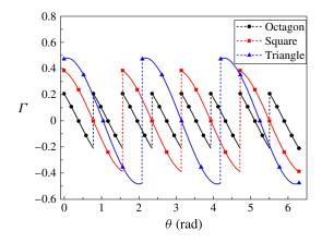
FIGURE 16. (Colour online) Normalized circulation  $\Gamma$  deposited per unit length along the initial interface boundaries for cross-sections of an octagon, a square and an equilateral triangle. The circulation is normalized by a constant which has a unit of velocity, i.e.  $a_0/\sqrt{\gamma} = 278 \text{ m s}^{-1}$ .
