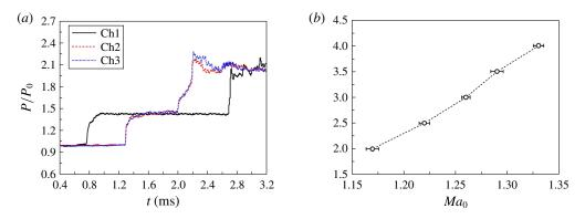
FIGURE 4. (Colour online) (a) Pressure histories of transducers Ch1–Ch3 mounted on the sidewall of the driven section for  $Ma_0 = 1.17$ . (b) Experimental measurements showing the pressure ratio between the driver and the driven sections versus the value of  $Ma_0$ .
