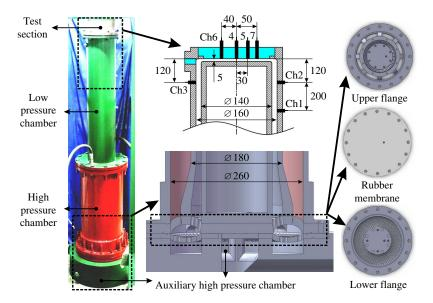
FIGURE 1. (Colour online) Photograph of the vertical annular diaphragmless shock tube and its detailed structures (unit: mm), designed following a principle similar to that presented in Hosseini *et al.* (2000).
