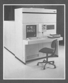
The Model 4175 Rutherford Backscattering Surface Analyzer is a compact, easy to operate instrument, designed for routine surface and depth characterization of thin films and solid materials. Rutherford Backscattering provides:
