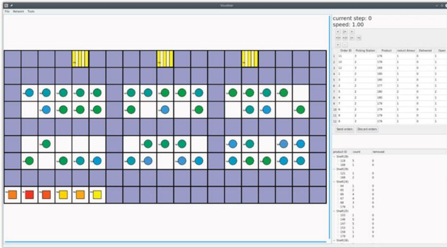
Fig. 1. Exemplary *asprilo* screenshot: The main window gives a warehouse layout; no plan is loaded. Picking stations are represented by striped yellow squares, shelves by solid circles, and robots by solid squares. Highways are brought out in purple. The side windows provide controls for plan animation, and give details about the current orders and the warehouse inventory.
