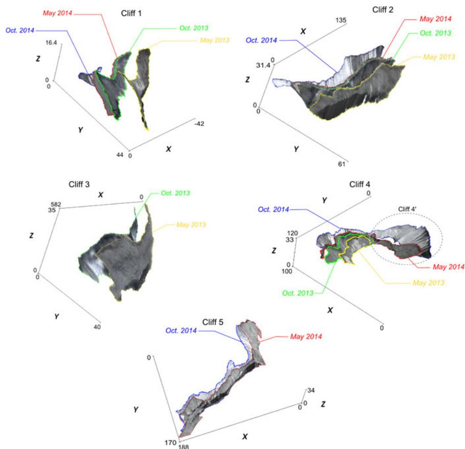
**Fig. 9.** Evolution of the cliffs between May 2013 and October 2014. The X, Y and Z coordinates are in meters with arbitrary origins. X and Y correspond to the easting and northing, respectively. All the TINs from which these figures are produced are shifted to the October 2014 base to correct for the ice flow.
