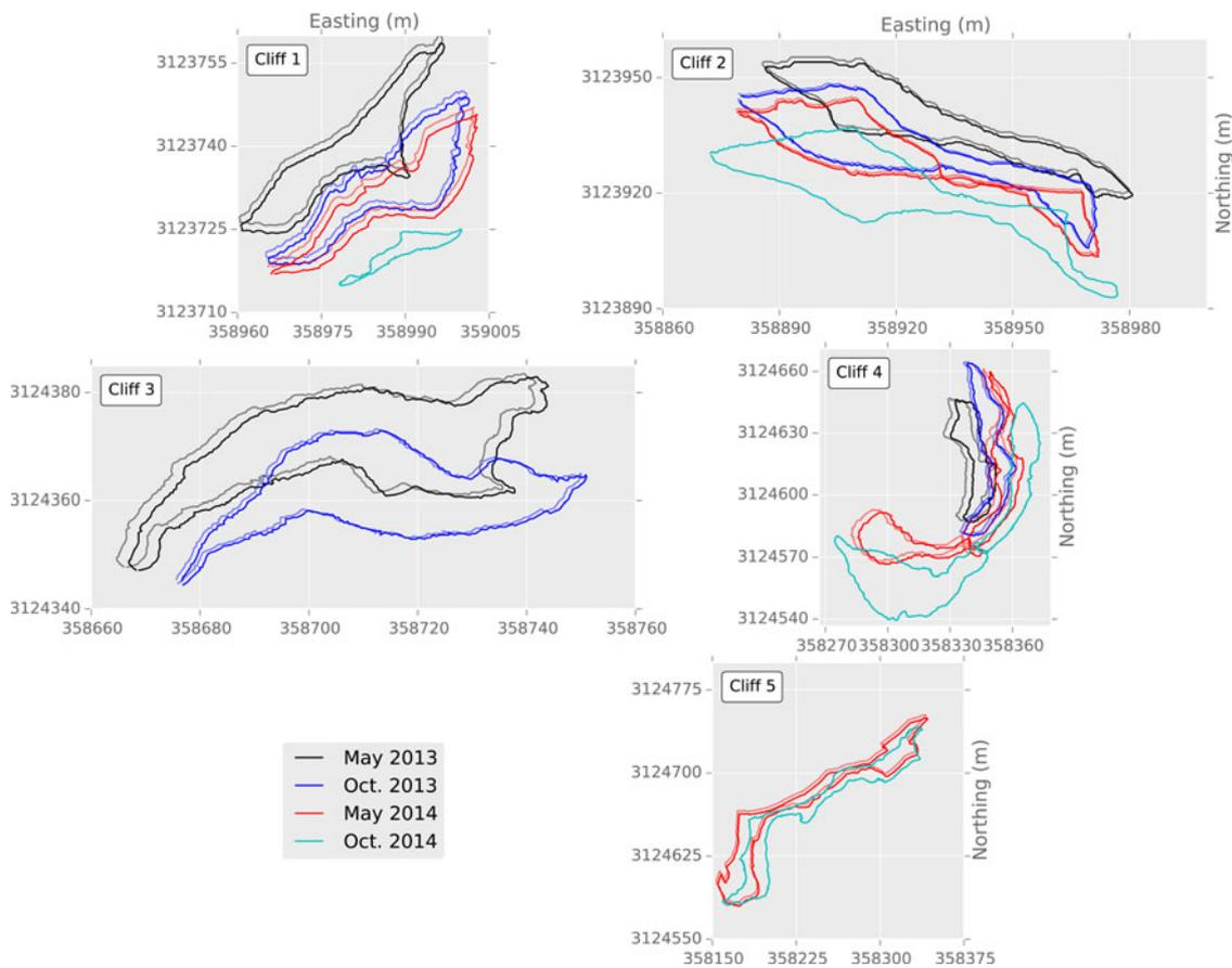
**Fig. 3.** Cliff outlines from May 2013 to October 2014. The light coloured outlines are the original cliff outlines and the darker outlines are after correction for the glacier flow according to the October 2014 base. All the coordinates are in UTM 45N/WGS84 system (m). Note the difference in the horizontal scale.
