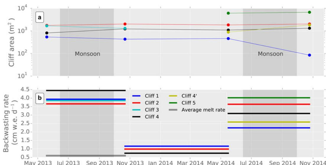
**Fig. 7.** Area change (a) and backwasting rate (b) of all cliffs as a function of time. The backwasting rate is defined as the volume change between  $t_1$  and  $t_2$  divided by the number of days and the mean cliff area. The average melt rate (grey) is from Immerzeel and others (2014). Note that the y-axis for the upper panel has a logarithmic scale. Shaded areas in both panels indicate the monsoon period (15 June–30 September).
