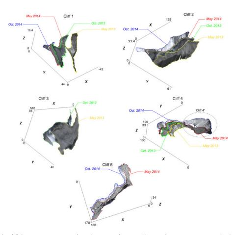
Fig. 9. Evolution of the cliffs between May 2013 and October 2014. The X, Y and Z coordinates are in meters with arbitrary origins. X and Y correspond to the easting and northing, respectively. All the TINs from which these figures are produced are shifted to the October 2014 base to correct for the ice flow.
