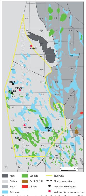
Fig. 3. Map of the study area showing the distribution of major gas fields and the major structural units. The wells used in the study are indicated. Wells used for 1D extractions used for burial history, temperature and maturity analysis are given the red colour.
