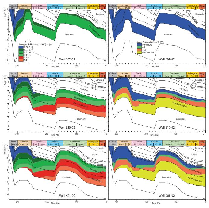
Fig. 10. Modelled maturity (left) and hydrocarbon generation (right) history for the major source rock units in thee well extractions. The modelled hydrocarbon generation is based on the applied generation kinetics for each source rock (Pepper & Corvi, 1995 TIII, TII).
