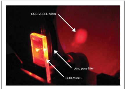
Photographic image of a red colloidal quantum dot, vertical-cavity surface-emitting laser (CQD-VCSEL) showing a spatially well-defined output beam, which is collinear with the pump beam. Reproduced with permission from *Nat. Nanotechnol.* **7** (2012) DOI: 10.1038/nnano.2012.61; p. 335. © 2012 Macmillan Publishers Ltd.
