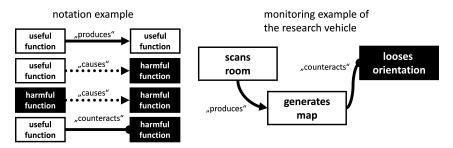
Figure 6. Relation-oriented function model
