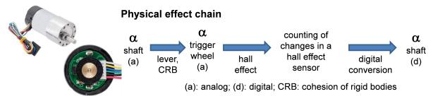
Figure 7. Physical effect chain motor encoder of the research vehicle
