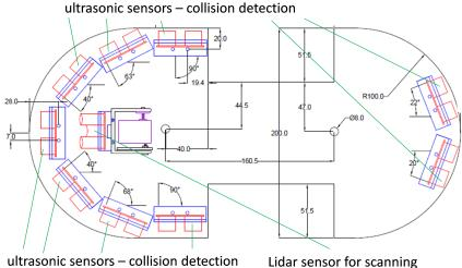
Figure 8. Location of sensors on the vehicle
