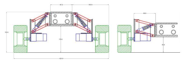
Figure 4. Chassis of the research vehicle
