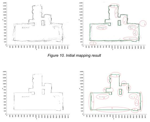
Figure 11. Mapping result after filtration
