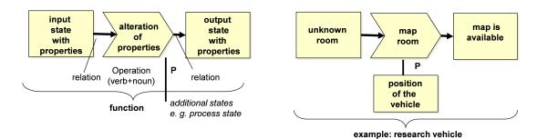
Figure 5. Flow-oriented function model
