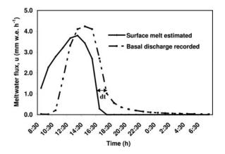
Fig. 5. Surface snowmelt estimated and discharge recorded by the lysimeter at Patsio field station on 23 April 2008.
