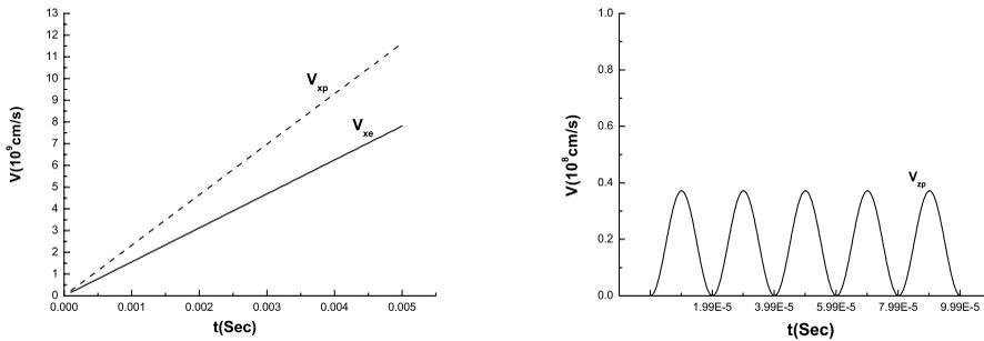
**Figure 1.** The time evolution of proton and electron velocity trajectory for  $B_0 = 200G$ ,  $B_y = -40G$ ,  $B_z = 1G$ ,  $v_p = -5 \times 10^8 \text{ cm/s}$ ,  $d = 2 \times 10^4 \text{ cm}$ , and  $G_e > 0$ ,  $G_p > 0$  (a)  $v_{xe}$  and  $v_{xp}$ , (b)  $v_{zp}$ .
