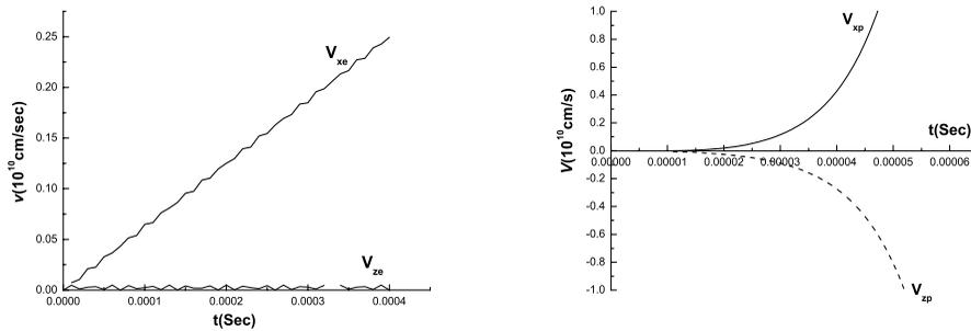
**Figure 2.** The time evolution of proton and electron velocity trajectory for  $B_0 = 200G$ ,  $B_y = -20G$ ,  $B_z = 1G$ ,  $v_p = -5 \times 10^8 \text{ cm/s}$ ,  $d = 2 \times 10^4 \text{ cm}$ , and  $G_e > 0$ ,  $G_p < 0$  (a)  $v_{xe}$  and  $v_{ze}$ , (b)  $v_{xp}$  and  $v_{zp}$ .
