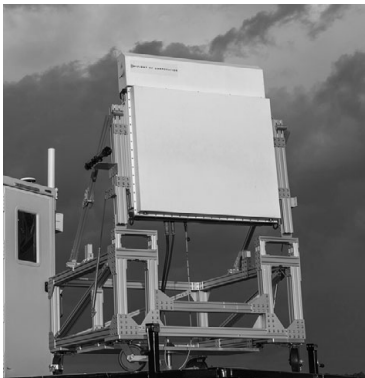
Figure 2.10 An X-band radar system using a planar electronically scanned antenna. Image courtesy of the Raytheon Technologies.
