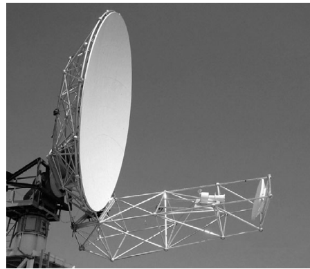
(b) Dual offset Gregorian (CSU-CHILL ©CSU)
