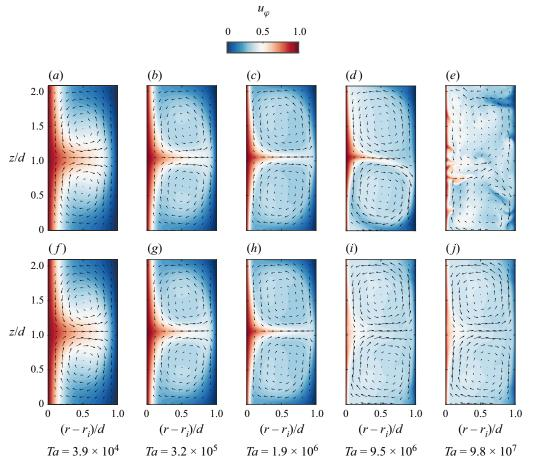
Figure 2. (a-e) Instantaneous snapshots of the azimuthal flow field (arrows denote  $u_r$ ,  $u_z$ ) for various Ta. (f-j) Corresponding time-averaged velocity fields. Here, the flow regimes are (a-c) Taylor vortex flow, (d) wavy vortex flow and (e) turbulent Taylor vortex flow.
