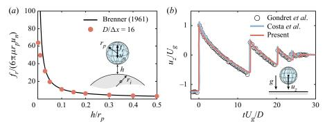
Figure 11. (a) Normalised force exerted on a sphere approaching a cylinder versus the shortest distance between the geometries. The radius ratio is set to  $r_i/r_p = 200$ . The theoretical prediction is from Brenner (1961). (b) A spherical particle falling on a flat plate at Ga = 130.4 and density ratio  $\rho_p/\rho_f = 8.34$ . The results are compared with experimental data reported in Gondret *et al.* (2002) and numerical results from Costa *et al.* (2015).
