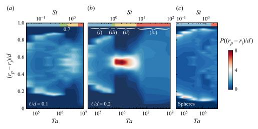
Figure 4. Joint p.d.f. of the particle normalised radial position versus Ta. Particles with size ratio  $(a) \ell/d = 0.1$  and  $(b) \ell/d = 0.2$ , and (c) spheres with identical volume to ellipsoids with  $\ell/d = 0.2$ . For reference, the modes addressed in § 4.1 are indicated with (i)–(iv) in the coloured top bar and the colour coding corresponds to the one used in figures 3 and 6.
