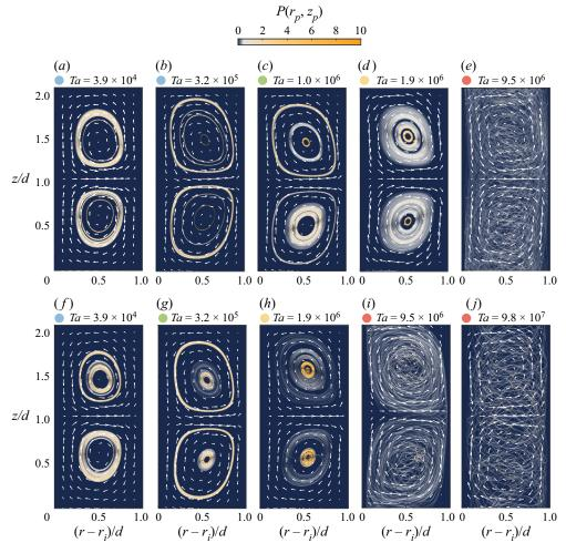
Figure 3. Probability density function of the particle distribution. The average is taken over time and azimuthal direction. (a-e) Particles of size  $\ell/d = 0.1$  and (f-j) particles of  $\ell/d = 0.2$ . The coloured circles on top of the contour plots denote distinguishable regimes of particle dynamics, which correspond to those in figures 4 and 6.
