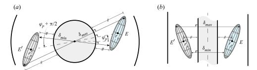
Figure 10. Overview of a particle and its ghost particle for two different configurations (not to scale). Here  $\delta_{\min}$  and  $\delta_{\max}$  are used to calculate the shortest and longest distance between particle E to the inner and outer cylinder, respectively. (a) Top view and (b) side view.
