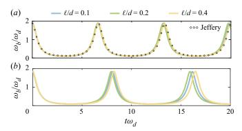
Figure 12. Curvature effects related to particle size. The rotational velocity  $\omega_b$  of a single pinned (where  $u_{\varphi}=0$ ) particle is tracked. The quantity is normalised with  $\omega_d=u_w/d$ , with  $u_w$  the wall velocity and d the gap width. (a) Plane Couette flow and (b) TC flow. For comparison, the result derived by Jeffery is included (Jeffery 1922).
