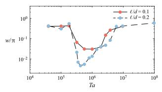
Figure 7. Width, w, of the p.d.f.  $P(\theta_7)$  versus Ta. The definition of w is sketched in figure 5.
