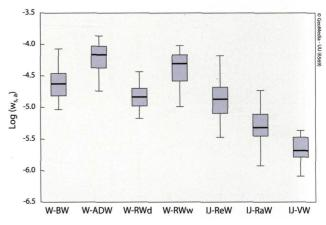
Fig. 5. Apparent settling velocity  $(\omega_{s,a})$  for all floodplains. The apparent settling velocity is a proxy for the trapping efficiency of a floodplain.
