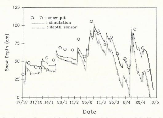
Fig. 4. Comparison between observed and simulated snow depth. ..., snow depth measured automatically with an ultrasonic sensor; o, snow depth deduced from the pit observations; —, simulated snow depth.
