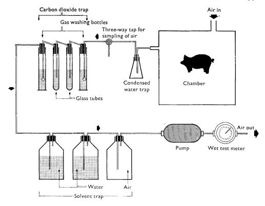
Fig. 1. Apparatus used to collect  ${}^{14}\text{CO}_2$  in ethanolamine-ethylene glycol monoethyl ether (1:2, v/v) from pigs which had received a dose of  ${}^{14}\text{C}$ -labelled amino acid.  $\blacklozenge$ , Direction of flow.
