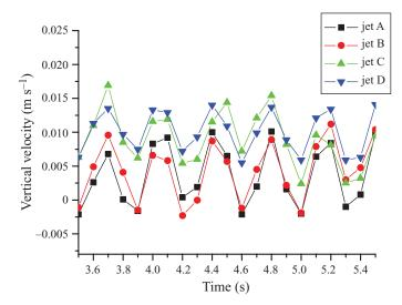
FIGURE 10. Jet oscillations at a forcing frequency of 160 Hz and a forcing acceleration of  $120 \text{ m s}^{-2}$ . The data show simultaneous measurements of the vertical velocities at four symmetrical points close to the four strongest vibrating locations A, B, C and D.
