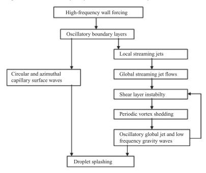
FIGURE 17. Schematic of possible excitation mechanisms for gravity wave generation and droplet splashing.
