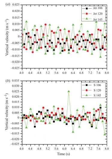
FIGURE 14. Jet and free surface velocities with increasing forcing accelerations for a forcing frequency of 160 Hz. (a) Jet velocities at three forcing accelerations of 106, 120 and 145 m s<sup>-2</sup>. (b) Free surface velocities at three forcing accelerations of 106, 120 and 145 m s<sup>-2</sup>. The jet velocities were measured at point B in figure 8(b) while the free surface velocities were measured at the centre of the free surface.
