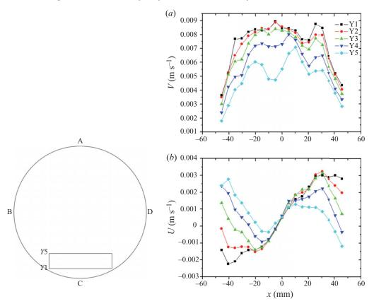
FIGURE 9. Jet profiles and velocity distributions in the streaming and cross-flow directions at a forcing frequency of 160 Hz and a forcing acceleration of  $120 \text{ m s}^{-2}$ . The flow conditions are the same as in figure 8. (a) Velocity distributions in the streaming direction. (b) Velocity distributions in the cross-flow direction. X is the distance from the centre of the cylinder and Y is the distance from the wall. U is along the X direction and V is along the Y direction.
