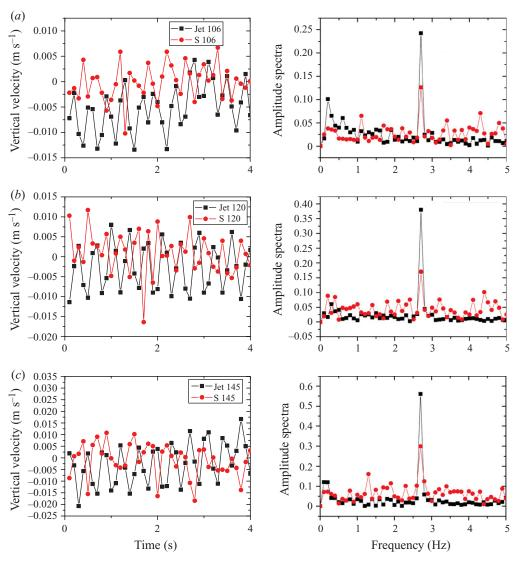
FIGURE 15. Phase and spectral relations between the jet and the free surface at a forcing frequency of 160 Hz. (a), (b) and (c) correspond to forcing accelerations of 106, 120 and  $145 \text{ m s}^{-2}$ , respectively.
