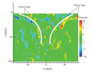
FIGURE 11. Series of vortex rings shed around the jets (shown by the white arrows) due to the Kelvin–Helmholtz instability. The forcing frequency is 160 Hz and the forcing acceleration is  $120 \text{ m s}^{-2}$ .
