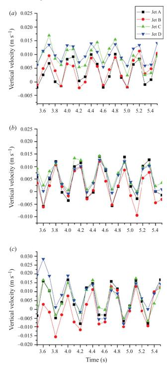
FIGURE 16. Phase relations of the four antinode jets at a forcing frequency of 160 Hz where (a), (b) and (c) correspond to forcing accelerations of 106, 120 and 145 m s<sup>-2</sup>, respectively.
