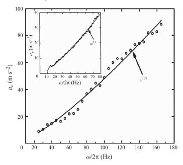
FIGURE 7. Critical acceleration for droplet ejection in water in a circular Plexiglas container with  $a_c = 0.13226 \ (\omega/2\pi)^{1.28}$  for frequencies in the capillary range. The inset shows the results of Goodridge, Shi & Lathrop (1996).
