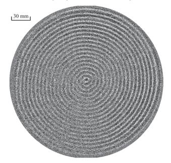
FIGURE 2. Photograph of the fluid surface at low-amplitude excitation. The waves are observed to propagate from the edge to the centre for an excitation frequency of 48.5 Hz. The bright lines correspond to wave crests while the dark lines correspond to wave troughs.
