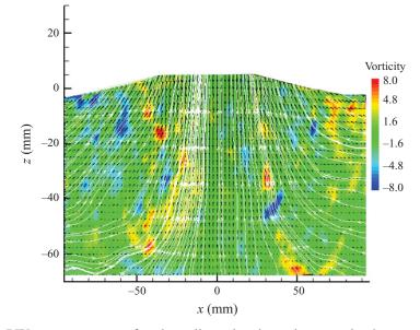
FIGURE 13. PIV measurements of a three-dimensional gravity wave in the container during the rising stage at a forcing frequency of 160 Hz and a forcing acceleration of  $170 \text{ m s}^{-2}$ . The dark arrows represent the velocity vectors, the colour contours represent the vorticity field for the (0, 1) mode low-frequency three-dimensional gravity wave, and the white curved arrows represent the streamlines.
