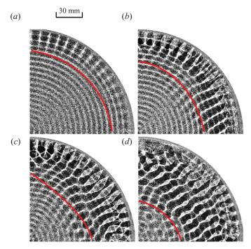
FIGURE 3. Evolution of azimuthal waves with increasing forcing amplitude. The wall acceleration (amplitude) was increased in this figure from 5.9 to  $12.1 \text{ m s}^{-2}$  (*a*)–(*d*) with an excitation frequency of 48.5 Hz. The upper region of the red curve indicates where the azimuthal waves emerge. With increased forcing amplitude, the influenced regions grow inwards and the interactions between the circular waves and the azimuthal waves intensify.
