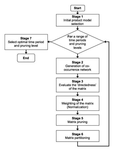
Fig. 2. Process of automatically generating design structure matrices.
