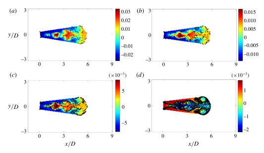
FIGURE 10. Vortex ring CSC, for particles introduced at nozzle exit plane while vortex ring is forming, calculated over the time interval  $t^* = [8.0, 10.2]$ : (a) 150 particles, (b) 300 particles, (c) 600 particles and (d) 2400 particles.
