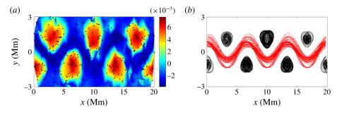
FIGURE 5. Bickley jet: (a) CSC contours overlaid with dots indicating final particle positions, 480 particles,  $t = [0, 3456 \times 10^3]$  s; and (b) particle tracks for particles with highest (black) and lowest (red) CSC values.
