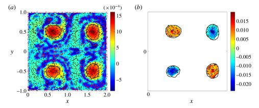
FIGURE 3. Unsteady quadruple gyre,  $\epsilon = 0.1$ , A = 0.1, T = [2.5, 42.5] and 3000 total particles. (a) CSC; black dots show final locations of particles that remained in their initial quadrant, and red dots show final locations of particles that switched quadrants during the coherent structure calculation time interval. Black lines trace contours of CSC = 0.0009. (b) CSC, algorithm applied recursively only to particles whose initial CSC value was greater than 0.0009.
