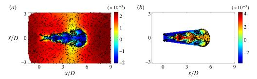
FIGURE 11. Vortex ring CSC, calculated over the time interval  $t^* = [8.0, 10.2]$ : (a) 1200 particles initiated randomly in full domain at  $t^* = 0$  and 1200 particles introduced at nozzle exit plane during vortex ring formation time,  $t^* = [0.04, 8.4]$ ; and (b) 1200 particles introduced at nozzle exit plane during vortex ring formation time,  $t^* = [0.04, 8.4]$ .
