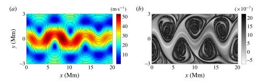
FIGURE 4. Bickley jet: (a) velocity magnitude with sample streamlines; and (b) FTLE field, calculated over the time interval  $t = [0, 3456 \times 10^3]$  s using 48 000 particles.
