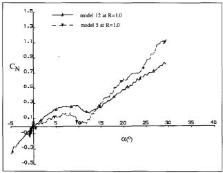
Figure 9.  $C_N$  plotted against incidence for ramp-down motion at r = -0.016. Model 12 and model 5 at R = 1.0.
