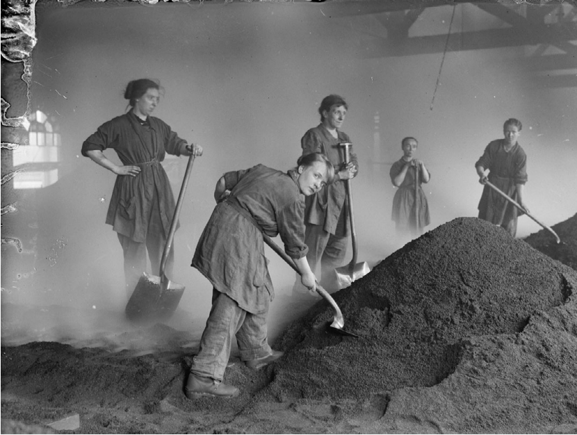
Figure I.2 Female workers feeding the charcoal kilns for refining sugar in the Glebe Sugar Refinery, Greenock. Photo by George P. Lewis for the Ministry of Information, November 1918. Imperial War Museum Q 28350.
