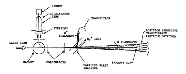
Figure 2. Schematic of Apparatus as Used for  $\operatorname{H}_2^+$  Photodissociation Experiment.
