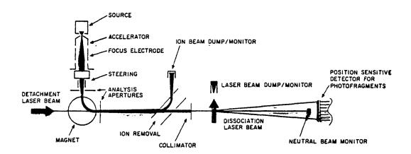
Figure 1. Schematic of Apparatus.
