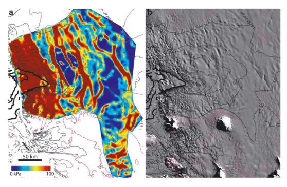
**Fig. 6.** (a) Inversion of basal shear stress calculated using viscous bed model for Thwaites Glacier and (b) MOA image. Glacier extents are indicated by the contours of glacier speed:  $50 \,\mathrm{m\,a^{-1}}$  contour (purple),  $100 \,\mathrm{m\,a^{-1}}$  contours up to  $900 \,\mathrm{m\,a^{-1}}$  (thin black), and  $1000 \,\mathrm{m\,a^{-1}}$  contours (thick black).
