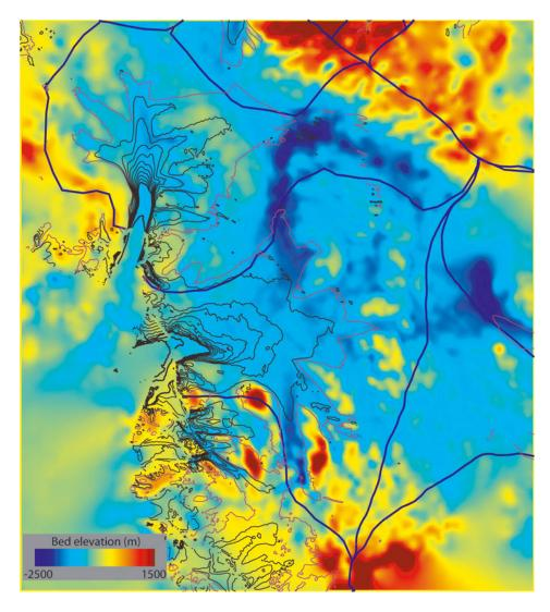
**Fig. 2.** Bed elevation for Pine Island and Thwaites Glaciers (Vaughan and others, 2006; Holt and others, 2007). Glacier extents are indicated by the contours of glacier speed:  $50 \text{ m a}^{-1}$  contour (purple),  $100 \text{ m a}^{-1}$  contours up to  $900 \text{ m a}^{-1}$  (thin black), and  $1000 \text{ m a}^{-1}$  contours (thick black).
