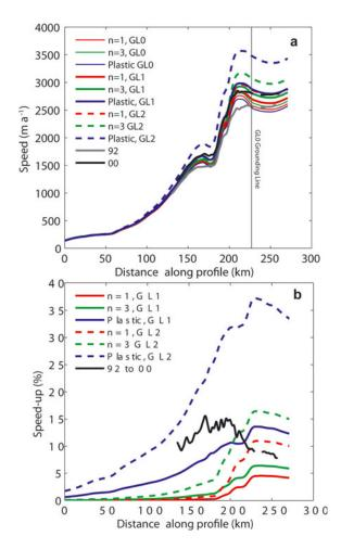
**Fig. 8.** (a) Modelled speed using different bed models (color) for the reference models (GL0) and grounding line retreats of 2.9 (GL1) and 5.2 (GL2) km. Also shown are InSAR-determined speeds from 1992 and 2000. (b) Speed-up expressed as percentage of the reference model speed (GL0) for grounding line retreat of 2.9 (GL1) and 5.2 (GL2) km.
