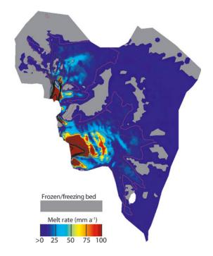
**Fig. 4.** Basal melt rates for Pine Island and Thwaites Glaciers. Glacier extents are indicated by the contours of glacier speed:  $50\,\mathrm{m\,a^{-1}}$  contour (purple),  $100\,\mathrm{m\,a^{-1}}$  contours up to  $900\,\mathrm{m\,a^{-1}}$  (thin black), and  $1000\,\mathrm{m\,a^{-1}}$  contours (thick black). Although the modelled values may be much higher, the color table saturates at  $100\,\mathrm{m\,m\,a^{-1}}$  to allow variation in regions of low melt to be distinguished.
