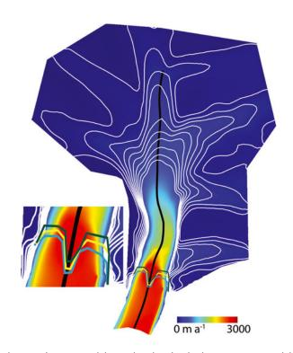
**Fig. 7.** Reference model speed (color) for the linear-viscous model. Speed is also shown with  $50\,\mathrm{m\,a^{-1}}$  white contours for values up to  $500\,\mathrm{m\,a^{-1}}$ . Inset shows the grounding line at the reference position (white) and after mean retreats of 2.9 and 5.2 km.
