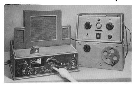
THIS MARCONI AUDIOMETER ASSEMBLY overcomes the familiar difficulties in pure tone audiometry of children. Subject reaction is encouraged by the provision of an interest-feature—a peepshow—which the child quickly learns to operate when the tone is audible, and which is inoperable when no tone is generated. The action of pressing the peepshow button constitutes involuntary acknowledgment of an
