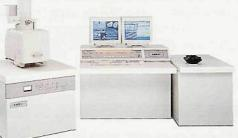
ized eucentric stage □ motorized 8" linear load lock for rapid sample exchange □ embedded computer control for all SEM functions
