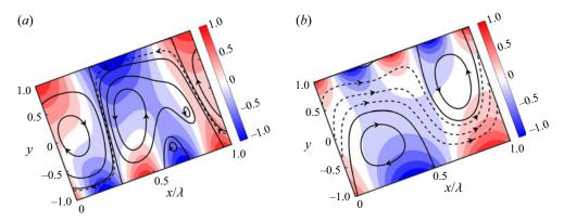
Figure 23. The flow and temperature fields when (a) CI = 0.5 and (b) CI = 2. All results correspond to the values  $\beta = \pi/4$ ,  $Ra_{p,L} = Ra_{p,U} = 200$  and  $\Omega = \pi/4$ . The solid lines identify streamlines within the separation bubbles while dashed lines identify streamlines within the stream tube. The temperature was normalized with  $\theta_{max} = Ra_{p,L}/2$ . The lower wall wavenumber is  $\alpha_L = 2$  in both cases.
