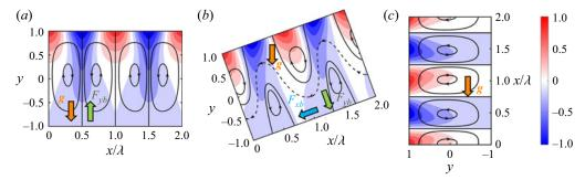
Figure 15. The flow and temperature fields for  $Ra_{p,U} = 400$ ,  $\alpha = 1.5$  and three inclinations angles (a)  $\beta = 0$ , (b)  $\beta = \pi/4$  and (c)  $\beta = \pi/2$ . Solid lines identify streamlines within the separation bubbles while dashed lines identify streamlines within the stream tube. The temperature was normalized with  $\theta_{max} = Ra_{p,U}/2$ . Thick arrows show direction of gravity and different components of the buoyancy force.
