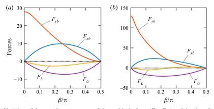
Figure 2. Variation of the *x*- and *y*-components of the total body force  $(F_{xb}, F_{yb})$  and the shear forces acting on the fluid at the lower  $(F_L)$  and upper  $(F_U)$  plates as functions of the inclination angle  $\beta$  for  $\alpha = 1.5$ , and (*a*)  $Ra_{p,L} = 400$  and (*b*)  $Ra_{p,L} = 1200$ .
