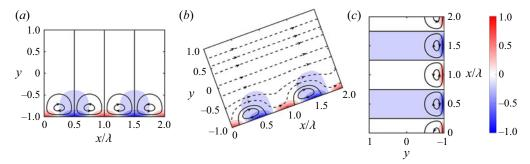
Figure 10. The flow and temperature fields for  $Ra_{p,L} = 400$ ,  $\alpha = 10$ , and for the three inclination angles (a)  $\beta = 0$ , (b)  $\beta = \pi/4$  and (c)  $\beta = \pi/2$ . Solid lines identify streamlines within the separation bubbles while dashed lines identify streamlines within the stream tube. The temperature was normalized with  $\theta_{max} = Ra_{p,L}/2$ .
