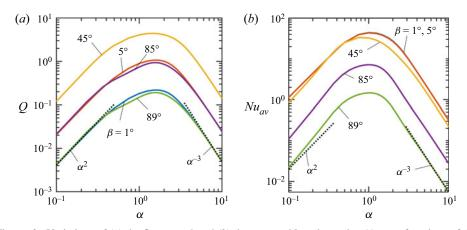
Figure 9. Variations of (a) the flow rate Q and (b) the average Nusselt number  $Nu_{av}$  as functions of the heating wavenumber  $\alpha$  for  $Ra_{p,L} = 400$ .
