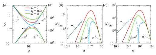
Figure 20. The variations of (a) the flow rate Q and (b, c) the average Nusselt number  $Nu_{av}$  as functions of the heating wavenumber  $\alpha$  when  $\beta = \pi/4$ . In (a)  $Ra_{p,L} = 200$ ,  $Ra_{p,U} = 100$  (left y-axis) together with  $Ra_{p,L} = 200$ ,  $Ra_{p,U} = 300$  (right y-axis). In (b)  $Ra_{p,L} = 200$ ,  $Ra_{p,U} = 100$  while in (c)  $Ra_{p,L} = 200$ ,  $Ra_{p,U} = 300$ . Dashed lines in (b,c) denote a change in sign.
