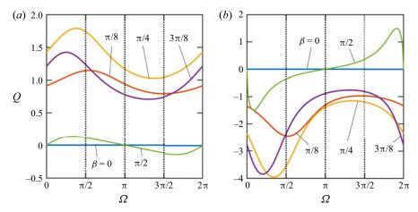
Figure 18. The variation of the flow rate Q as a function of the phase difference  $\Omega$  when  $Ra_{p,L} = 200$ ,  $\alpha = 1.5$ . In (a) the lower plate is hotter with  $Ra_{p,U} = 100$ ; in (b) the upper plate is the warmer ( $Ra_{p,U} = 300$ ).
