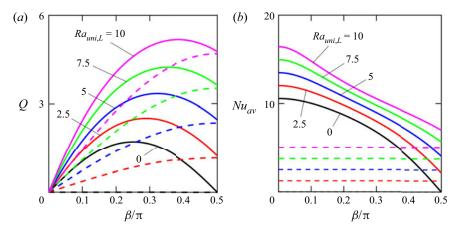
Figure 13. Illustration of the effects of uniform heating; (a) the variation of the flow rate Q and (b) the average Nusselt number  $Nu_{av}$  for various levels of uniform heating as functions of the inclination angle  $\beta$  when  $\alpha = 1.5$ . Solid lines denote results for combined uniform and periodic heating with  $Ra_{p,L} = 200$ . Dashed lines indicate the reference results for a purely uniform heating ( $Ra_{p,L} = 0$ ).
