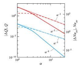
Figure 25. A comparison of the numerically and analytically determined flow rates Q and average Nusselt numbers  $Nu_{av}$  for the short-wavelength heating when  $Ra_{p,L} = 400$ ,  $\beta = \pi/4$ . The red lines refer to the flow rate:  $Q_n$  dashed line,  $Q_a$  – dotted line,  $|\Delta Q|$  – solid line. Blue colour refers to the Nusselt number:  $Nu_{av,n}$  – dashed line,  $Nu_{av,a}$  – dotted line,  $|\Delta Nu_{av}|$  – solid line.
