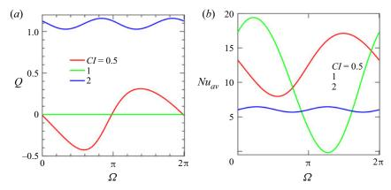
Figure 22. Variation of (a) the flow rate Q and (b) the average Nusselt number  $Nu_{av}$  as functions of the phase shift  $\Omega$  for three values of the commensurability index CI = 0.5, 1, 2, and for  $\beta = \pi/4$ ,  $Ra_{p,L} = Ra_{p,U} = 200$ . In all cases the wavenumber at the lower wall is  $\alpha_L = 2$ .
