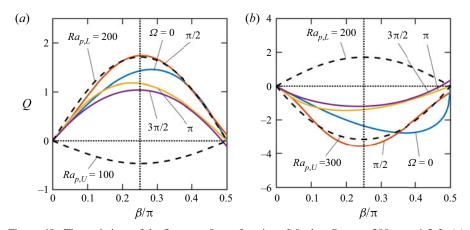
Figure 19. The variations of the flow rate Q as a function of  $\beta$  when  $Ra_{p,L} = 200$ ,  $\alpha = 1.5$ . In (*a*)  $Ra_{p,U} = 100$  while in (*b*)  $Ra_{p,U} = 300$ . Dashed lines show the values of Q generated by heating one plate only.
