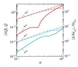
Figure 24. A comparison of the numerically and analytically determined flow rates Q and average Nusselt numbers  $Nu_{av}$  for the long-wavelength heating with  $Ra_{p,L} = 400$ ,  $\beta = \pi/4$ . The red lines refer to the flow rate with  $Q_n$  the dashed line,  $Q_a$  the dotted line and  $|\Delta Q|$  the solid line. The blue lines refer to the Nusselt number:  $Nu_{av,n}$  – dashed line,  $Nu_{av,a}$  – dotted line,  $|\Delta Nu_{av}|$  – solid line.
