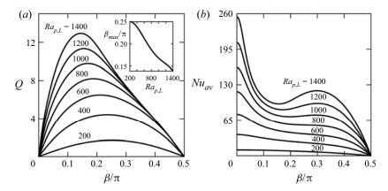
Figure 5. Variations of (a) the flow rate Q and (b) the average Nusselt number  $Nu_{av}$  as functions of the inclination angle  $\beta$  for  $\alpha = 1.5$  and for selected values of  $Ra_{p,L}$ . The inset graph in figure 5(a) shows the variation of the angle  $\beta_{max}$  corresponding to the maximum flow rate as a function of  $Ra_{p,L}$ .
