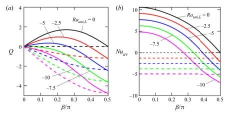
Figure 14. Illustrations of the effects of uniform cooling – variations of (a) the flow rate Q and (b) the average Nusselt number  $Nu_{av}$  for a selection of uniform cooling values as functions of the inclination angle  $\beta$  for  $\alpha = 1.5$ . Dashed lines provide reference results for a purely uniform cooling. Solid lines denote results for the combined uniform cooling and periodic heating with  $Ra_{p,L} = 200$ .
