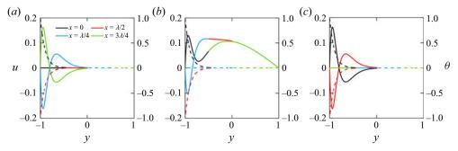
Figure 11. The profiles of the *u*-velocity component (solid lines) and the temperature  $\theta$  (dashed lines) as functions of *y* for  $Ra_{p,L} = 400$ ,  $\alpha = 10$  at four streamwise locations and the three inclinations angles (*a*)  $\beta = 0$ , (*b*)  $\beta = \pi/4$  and (*c*)  $\beta = \pi/2$ . Again, the temperature was normalized with  $\theta_{max} = Ra_{p,L}/2$ .
