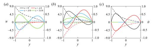
Figure 6. Distribution of the x-velocity component u (solid lines) and the temperature  $\theta$  (dashed lines) as functions of y for  $Ra_{p,L} = 400$ ,  $\alpha = 1.5$  and (a)  $\beta = 0$ , (b)  $\beta = \pi/4$  and (c)  $\beta = \pi/2$ ,  $\Omega = \pi$ . Temperature was normalized with  $\theta_{max} = Ra_{p,L}/2$ . The thin dotted horizontal line in (b) identifies the zero level in u and  $\theta$ .
