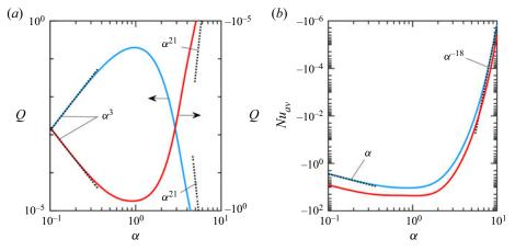
Figure 21. Variations in (a) the flow rate Q and (b) the average Nusselt number  $Nu_{av}$  in a vertical slot as functions of the heating wavenumber  $\alpha$ . Blue curves correspond to  $Ra_{p,L} = 200$ ,  $Ra_{p,U} = 100$ ,  $\Omega = \pi/2$ ; red curves correspond to  $Ra_{p,L} = 200$ ,  $Ra_{p,L} = 200$ ,  $Ra_{p,L} = 300$ ,  $\Omega = \pi/2$ .
