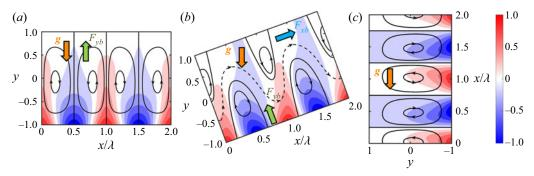
Figure 3. The flow and the temperature fields for  $Ra_{p,L} = 400$ ,  $\alpha = 1.5$  and (a)  $\beta = 0$ , (b)  $\beta = \pi/4$  and (c)  $\beta = \pi/2$ . Solid lines identify streamlines within the separation bubbles while dashed lines identify streamlines within the stream tube. The temperature was normalized with  $\theta_{max} = Ra_{p,L}/2$ . Solid arrows show direction of gravity and different components of the buoyancy force.
