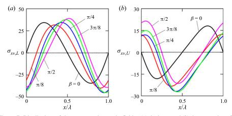
Figure 7. Distributions of shear stress acting on the fluid at (*a*) the lower and (*b*) the upper plates for  $Ra_{p,L} = 400$ ,  $\alpha = 1.5$ .
