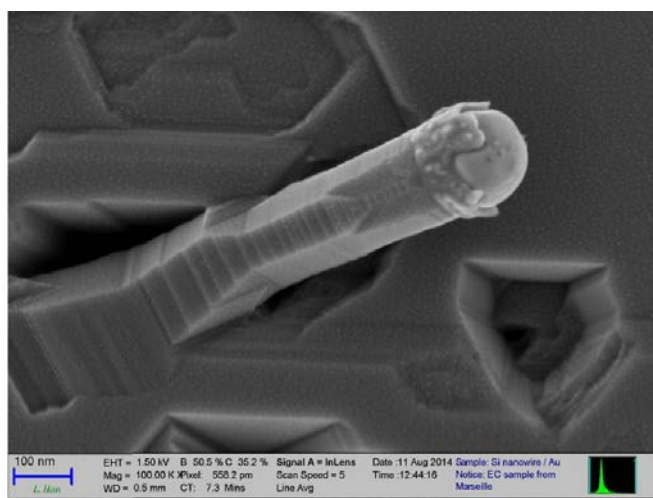
Figure 1. In-lens SE detector image of a Si NW clearly showing different facets and its fine structure on the surface. The surface sensitive imaging at 1.5 kV reveals highly resolved crystalline facets on the Si NW.
