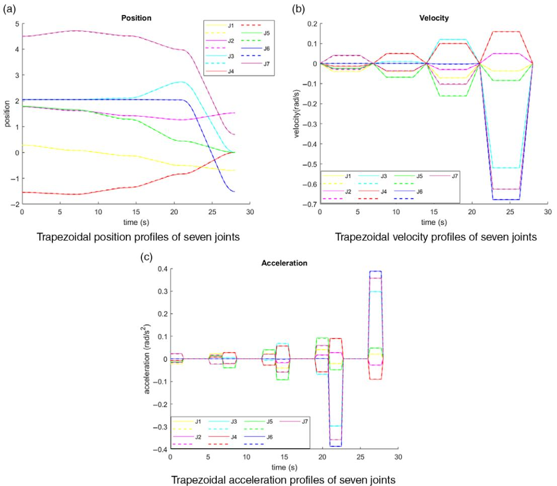
**Figure 6.** Trapezoidal position, velocity, and acceleration profiles of seven joints of the Kinova Gen3 robotic arm for the paths  $r_4$  (straight) and  $r_{14}$  (dashed).
