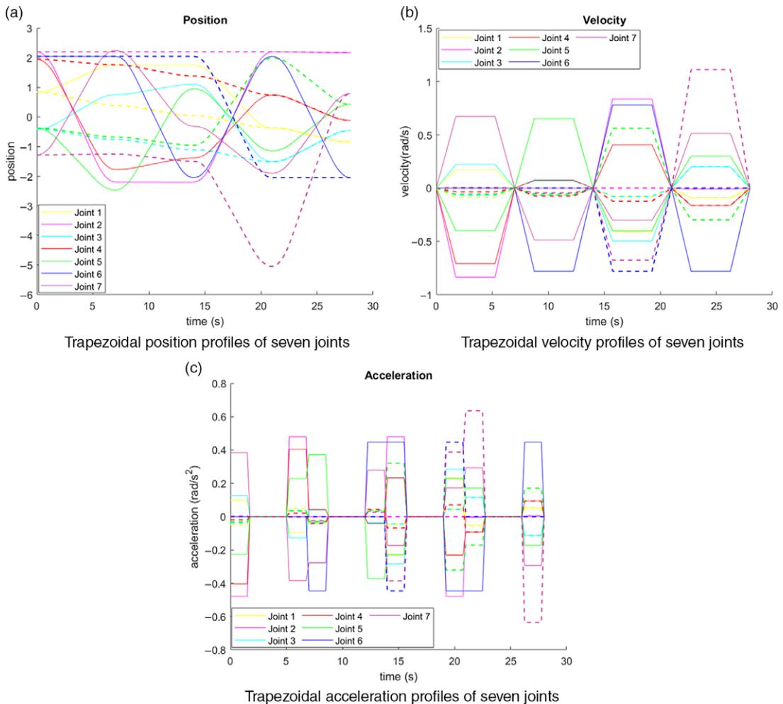
**Figure 12.** Trapezoidal position, velocity, and acceleration profiles of seven joints of the Kinova Gen3 robotic arm for the paths  $r_5$  (straight) and  $r_{15}$  (dashed).
