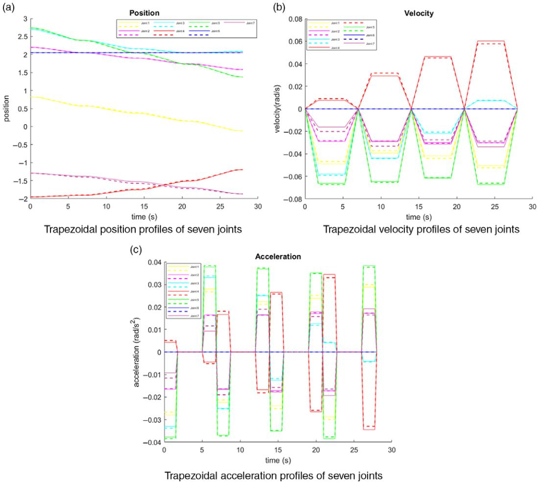
**Figure 9.** Trapezoidal position, velocity, and acceleration profiles of seven joints of the Kinova Gen3 robotic arm for the paths  $r_5$  (solid) and  $r_{15}$  (dashed).
