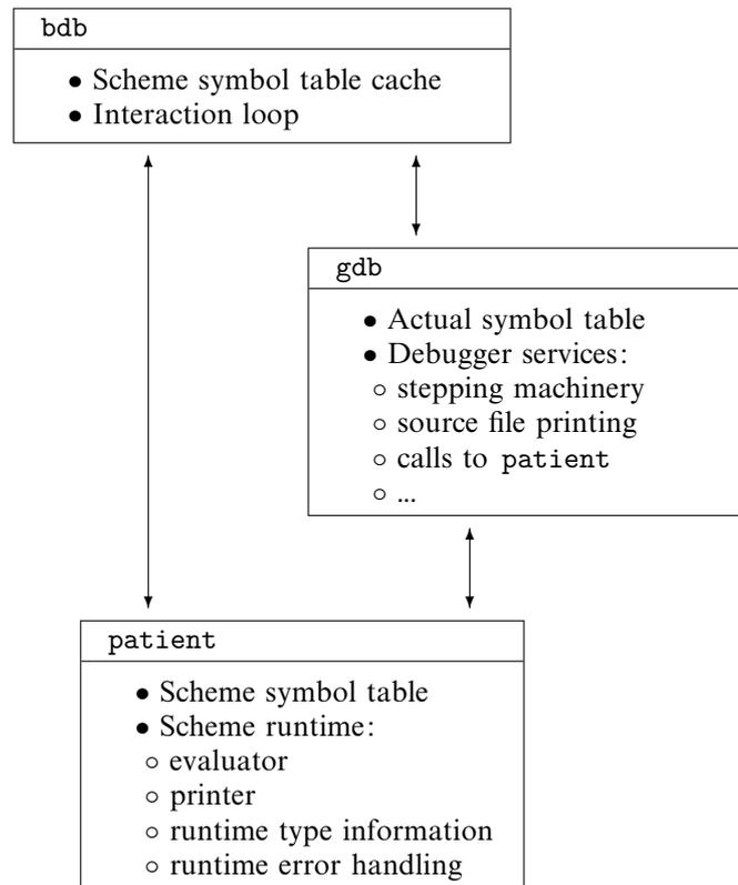
Fig. 7. The debugger architecture.
