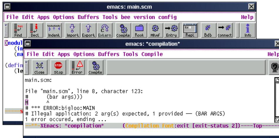
Scheme errors are reported in the source code. The compilation status window may be used to pop up a window displaying the culprit line of source code. This feature is common for C environments but unusual for Scheme environments. It requires a compiler that is able to find out source locations from its compilation abstract syntax tree. Section 6.3.1 presents an overview of the implementation of that feature.
