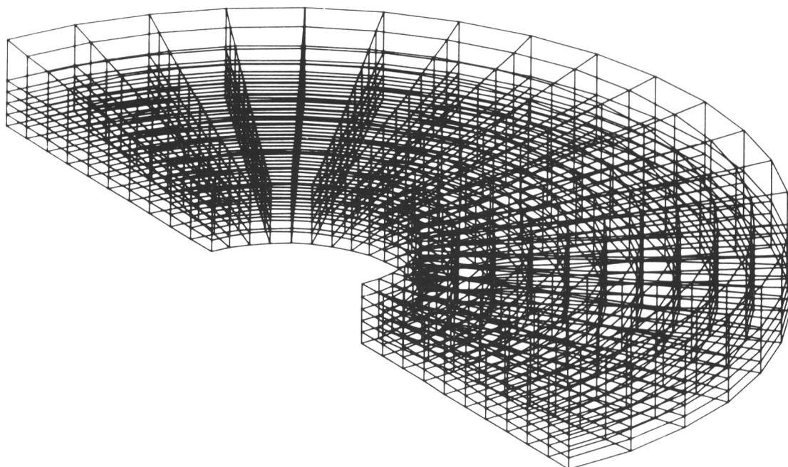
Fig. 3 MODEL BEING DEVELOPED TO DETERMINE EFFECT OF AXIAL AND RADIAL SUPPORTS
