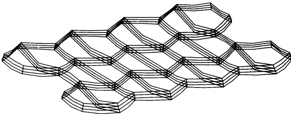
Fig. 8 DEFORMED SHAPE OF TOP SURFACE DUE TO FIGURING PRESSURE
