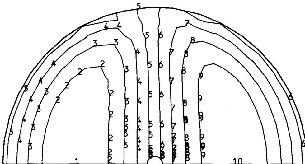
Fig. 5 CONTOUR MAP SHOWING DEFLECTIONS OF CORRECTOR LENS ELEMENT WITH TUBE VERTICAL
