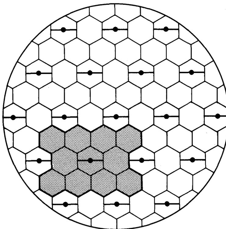
Fig. 6 CELLS AND SUPPORT LOCATIONS OF 1.8m HONEYCOMB MIRROR BLANK
