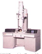
JEM-2010 Transmission Electron Microscope
